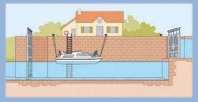
Once the boat or boats in the lock are secured, the lock keeper will close the gates.
