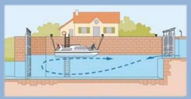
After closing the gates, the lock keeper will open the sluice gates and fill the lock with water. To keep the boat steady, the bow and stern lines must be kept tight during this time.
