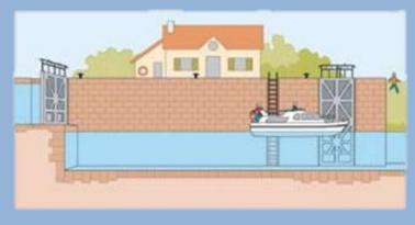
Once the water level in the lock has dropped to the level outside the lock, the lock keeper will open the gates. The bow and stern lines should be taken back onto the boat and the boat may then be driven slowly out of the lock.
