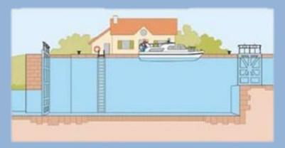
Once the lock is full, the lock keeper will open the lock gates. The bow and stern lines should be taken back onto the boat and the boat may then be driven slowly out of the lock.
