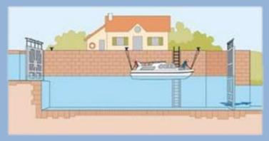
After closing the lock gates, the lock keeper will open the sluice gates and empty the lock of water. To keep the boat steady as the lock empties, the bow and stern lines must be kept tight during this time.
